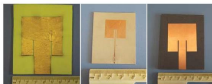
Figure 6.—Photograph of patch antenna on polyimide aerogel substrate (left), Rogers Duroid 6010 ( \epsilon_r = 10.2 ) (center); and Rogers Duroid 5880 ( \epsilon_r = 2.2 )(right) (Ref. 1).
